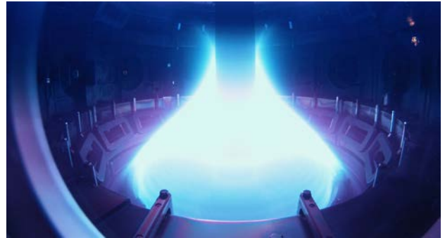
A plasma is contained in the MAST tokamak fusion experiment.
